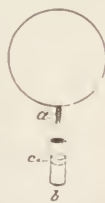
FIG. 45.— a , ring of metal tied with wire at a ; b , ferrule; c , plug put in before pouring in solder (Riley)
